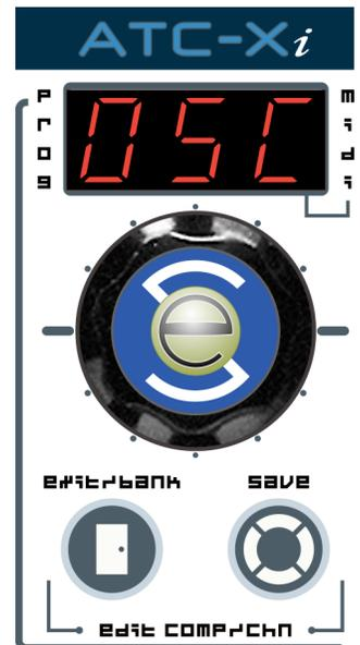
**To Save a patch:** To save a sound to the patch memory, press **save** once; the display will flash the current patch number, pressing **save** again will record it to its current location; to save the sound to a new location, rotate the encoder to the desired number, then press **save** once again.
