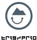
Selects the key triggering and note priority functions. Press once to access single or multiple triggering selections. Press again to access note priority selection. **Multiple triggering** is the re-triggering of the filter envelope with each note or keystroke; with single triggering the filter envelope is re-triggered only with staccato, or non-legato key strikes. **Note Priority** determines if while a holding note, any new note, or a lower note only, will be played next.
